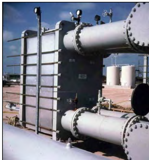
Power Generation Plant Auxiliary Cool Water Exchanger MODU-FLEX™ Model MFK201 - 20" ports Design Pressure: 150 PSIG Heat Transfer Area: ~ 12,000 ft 2
