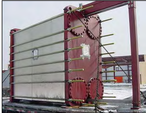
Mid-Atlantic Power Plant Auxiliary Cooling Water Heat Exchanger MODU-FLEX™ Model MFK200 - 20" ports Design Pressure: 150 PSIG Heat Transfer Area: ~ 13,000 ft 2
